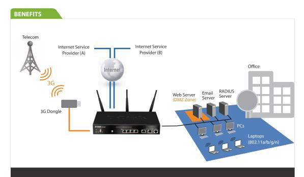
If you are running an e-commerce business and cannot afford to have any lost Internet connection, you can engage two Internet service providers and use the dual-WAN ports and 3G redundant features of the DSR series service router to provide seamless Internet redundancy. You can also set your e-commerce server in the DMZ zone with dedicate service provider line, if required, to ensure sufficient bandwidth for your customers.
